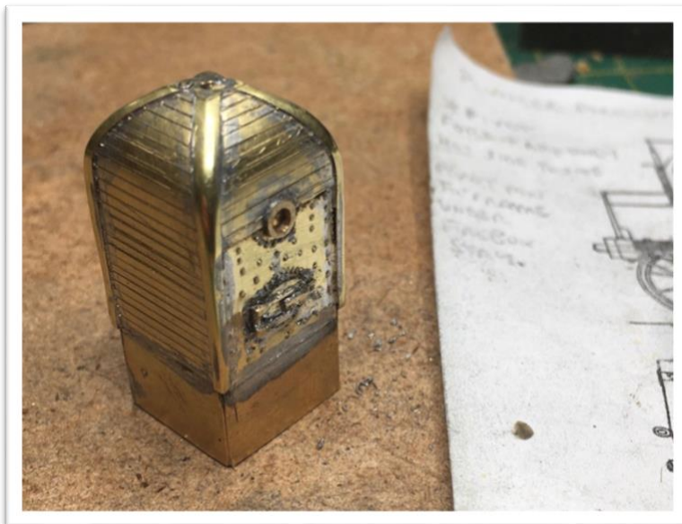
The exposed section of the firebox was cut away after assembly and a new piece of 10thou brass overlaid with brass foil pricked from the back to represent the many rivets was soldered in place.
