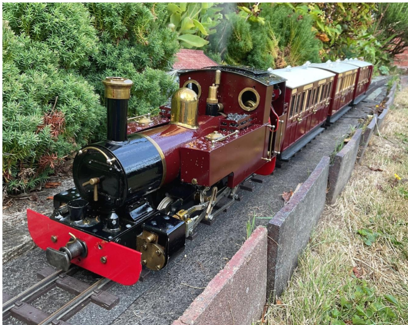
0-6-0 Lady Anne locomotive with a train of Brandbright turn of the century style kit built coaches. The oily water on the engine is a result of the boiler being topped up whilst in steam but overfilled.
