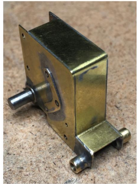
A new gearbox containing the Portescap gears. The L shaped strips on the side are retainers to keep the short gear shafts in place.
