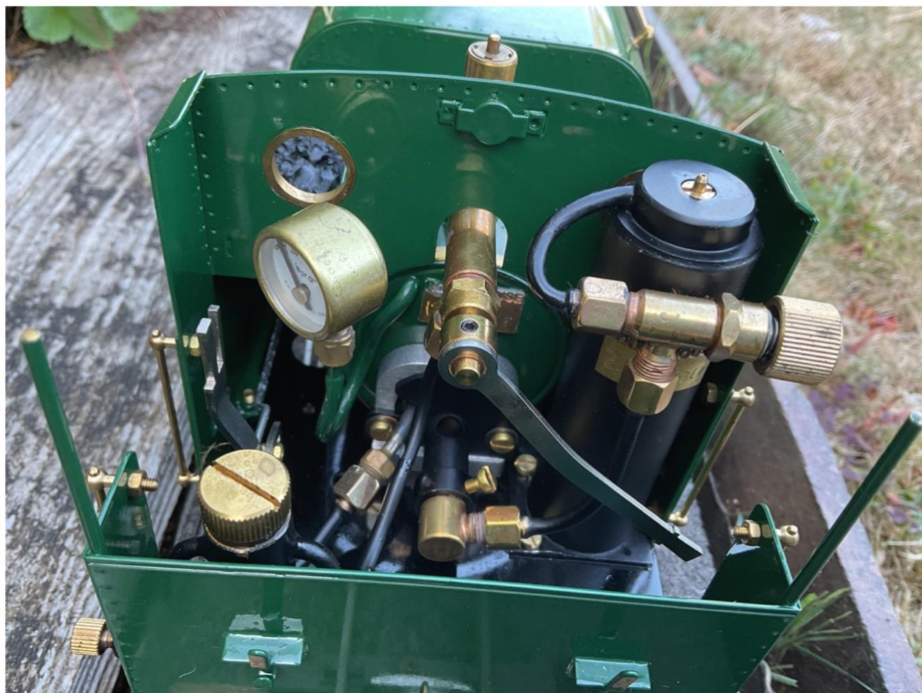
A view of Dylan's footplate showing the displacement lubricator, forward and reverse lever, pressure gauge, steam circuit pipework, gas burner, regulator and gas tank.
